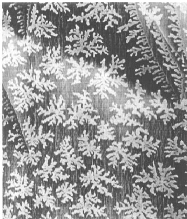
Figure 8. STM topograph of a 0.37 ML Au film on Ru(0001) deposited at room temperature ( 9300 \times 10\,300 \text{ \AA}^2 ). (Reprinted from ref 49. Copyright 1992 American Vacuum Society.)
